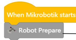
This block is to prepare robot with specific *library* and to configure pin numbers and pot numbers in and out for each sensor and output attached to the robot.
