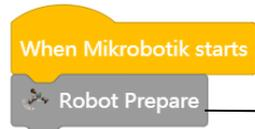
This block is to prepare robot with specific *library* and to configure pin numbers and pot numbers in and out for each sensor and output attached to the robot.
