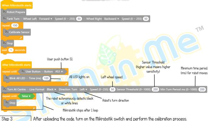
After uploading the code. turn on the Mikrobotik switch and perform the calibration process. After that. Mikrobotik will make a U-turn according to the set direction and will stop after detect the black line.
